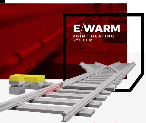
e-WARM is designed to prevent problems in the railway points, which occur due to snow and icing at adverse weather conditions. The system enables automatic operation with the help of its snow-ice and temperature sensors and ensures uninterrupted and safe railway operation.
